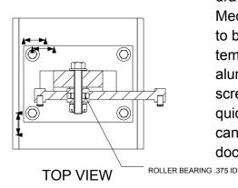
This schematic design concept was rapidly drawn using the Mechanical Engineering Mechanical Parts Library solution. In addition to basic drawing and annotation shapes, this template offers a set of stencils with steel and aluminum sections, bearings, nuts, bolts, screws, and so on, allowing the engineer to quickly assemble an accurate sketch, which can then be further refined as a design document or shop drawing.
